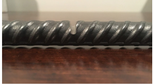
Rebar Sample: 1/2 Cut
