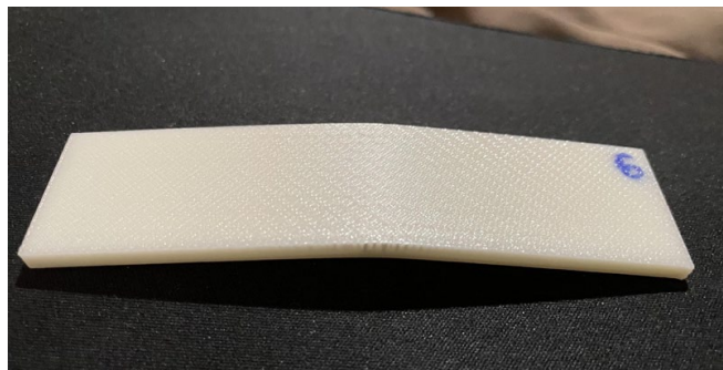
Figure 5. Sample 6 (45° orientation) after it underwent its 3-Point Bending test and a ductile failure mode.
